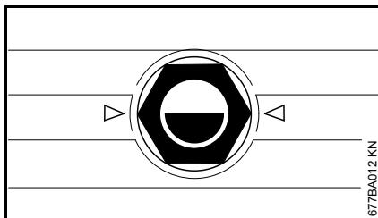
The oil level in the high-pressure pump and the gearbox (RB 402 PLUS only) must be checked at monthly intervals.
