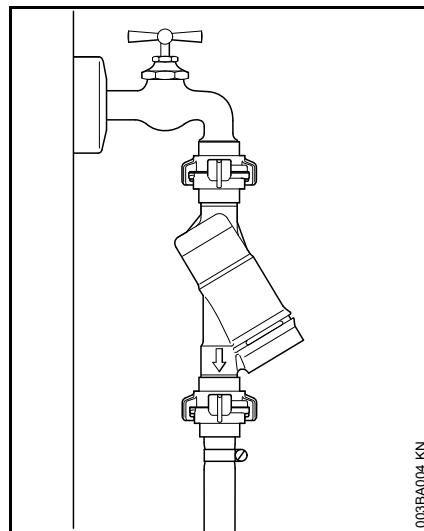
When hooking up to the drinking water main, a backflow preventer (in accordance with IEC/EN 60335-2-79) must be installed between the water tap and the hose.
